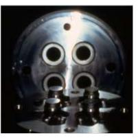
Solid dies may, on occasion, be used to produce hollow profiles by means of a fixed or floating mandrel. The use of a mandrel for extruding a hollow shape through a flat die usually involves the use of hollow billets, cylindrical source stock that may have been cast or bored. Piercing mandrels, however, do not require the use of cored billet.
