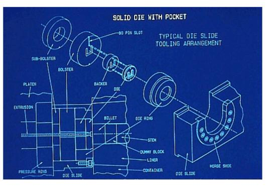
This diagram shows the components that typically make up a die slide, the tooling assembly, for a solid die.
