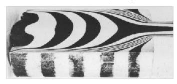
As heated aluminum is forced out of the container and through the die, the core of the billet flows more rapidly than the periphery, as illustrated by the dark banding in this photograph. The periphery, which is left behind as residue, is recycled for future use.
