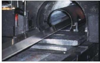
These photos show a new length of extrudate, just emerging from the press (left) and the production of a profile in progress (right).
