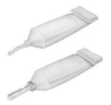
As suggested by these toothpaste tubes, the shape of the extrusion (profile) is determined by the shape of the opening (die).
